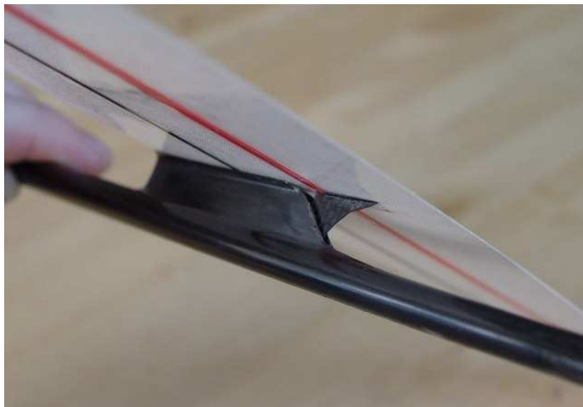
Fig. 2.5.: The elevator horn is hidden inside the pylon.
