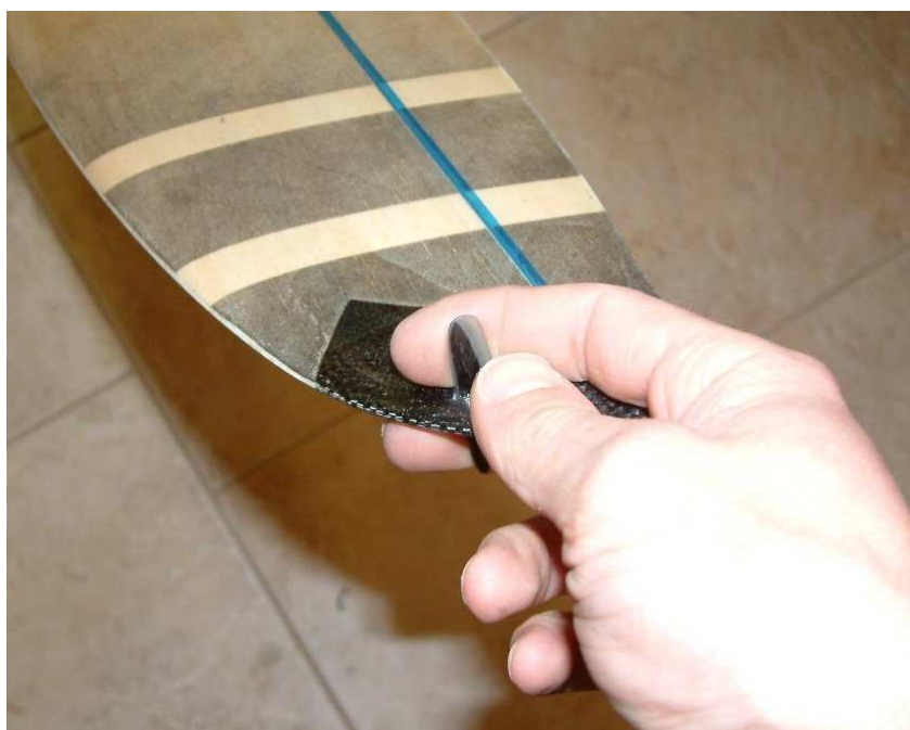
Fig. 3.1.: Only the fingertips of fore and middle finger grab the launch peg.
