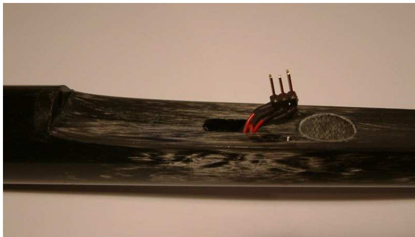
Fig. 2.3.: Servo plug in the fuselage made from 2.54 mm PCB header.
