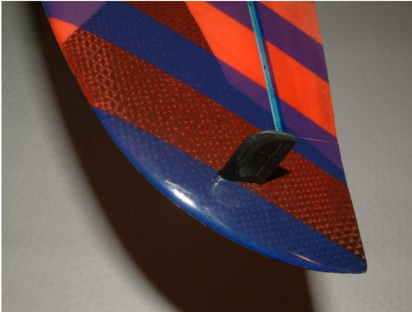
Fig. 2.13.: Glue in the launch peg with thin CA.
